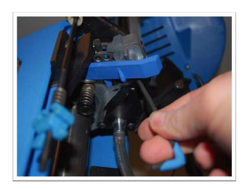
Using a 9/64" Allen Wrench start by removing the two screws that hold the original missed primer chute ramp (ski jump) to the platform. This may be easier done with the platform in the raised/handle down position. Lower the platform after you have removed the Primer chute ramp.
