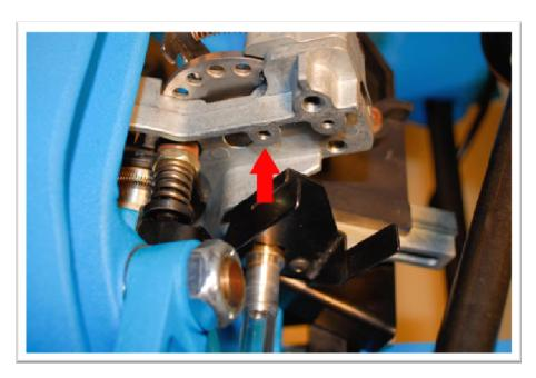
The new Primer Catcher will mount to the left side bolt hole of the original chute location.
