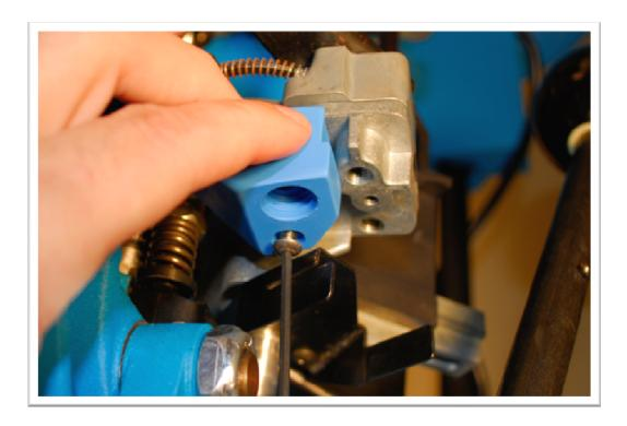
Insert the new supplied screw and using a 3/32" Allen tighten the screw to secure the new Primer Catcher to the platform. It might be a tight fit but the screw and allen should just clear the stock spent primer cup bracket.
