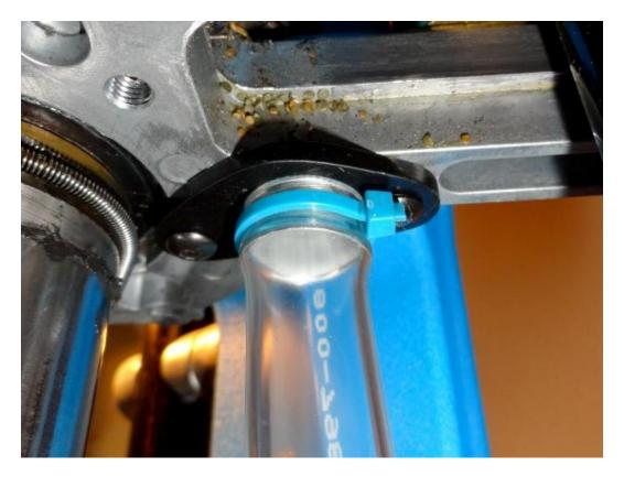
Next attach one end of the Hose to the Funnel and secure it with one of the small zip ties.
