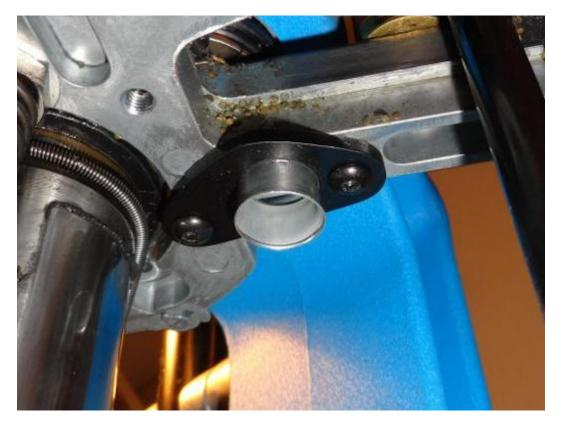
Using the supplied screws attach the new Funnel and Bracket in the position shown above.
