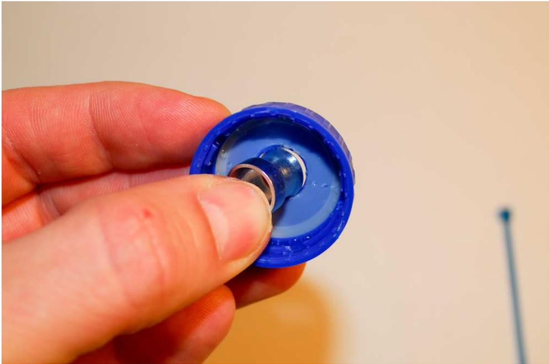
If using a soda bottle double check that the supplied cap fits your bottle before continuing. Insert the bottom hose fitting (the smaller of the two fittings) through the bottom of the cap, it might be a tight fit and inserting it at an angle and then snapping it in is usually the easiest method here.
